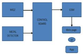
iot bomb detection model above figure shows different parts like gsm, arduino connected between ,web page ,metal detector,control board etc. It board
